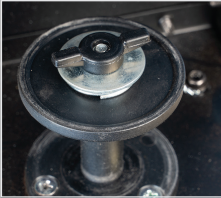
(1) Remove the spool retaining nut.
