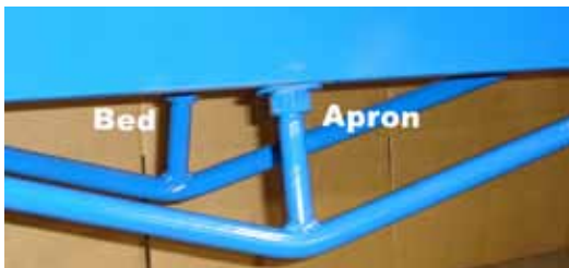
Apron & Bed Adjustment Nuts
