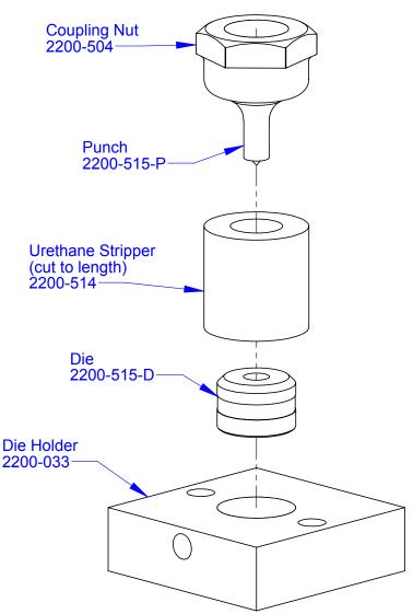
Urethane strippers generate high holding pressure on the blank and strip the blank cleanly from the punch.
